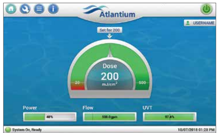
Atlantium's All-in-One (AiO) controller sets a new standard in precision, monitoring and operation of UV systems.
